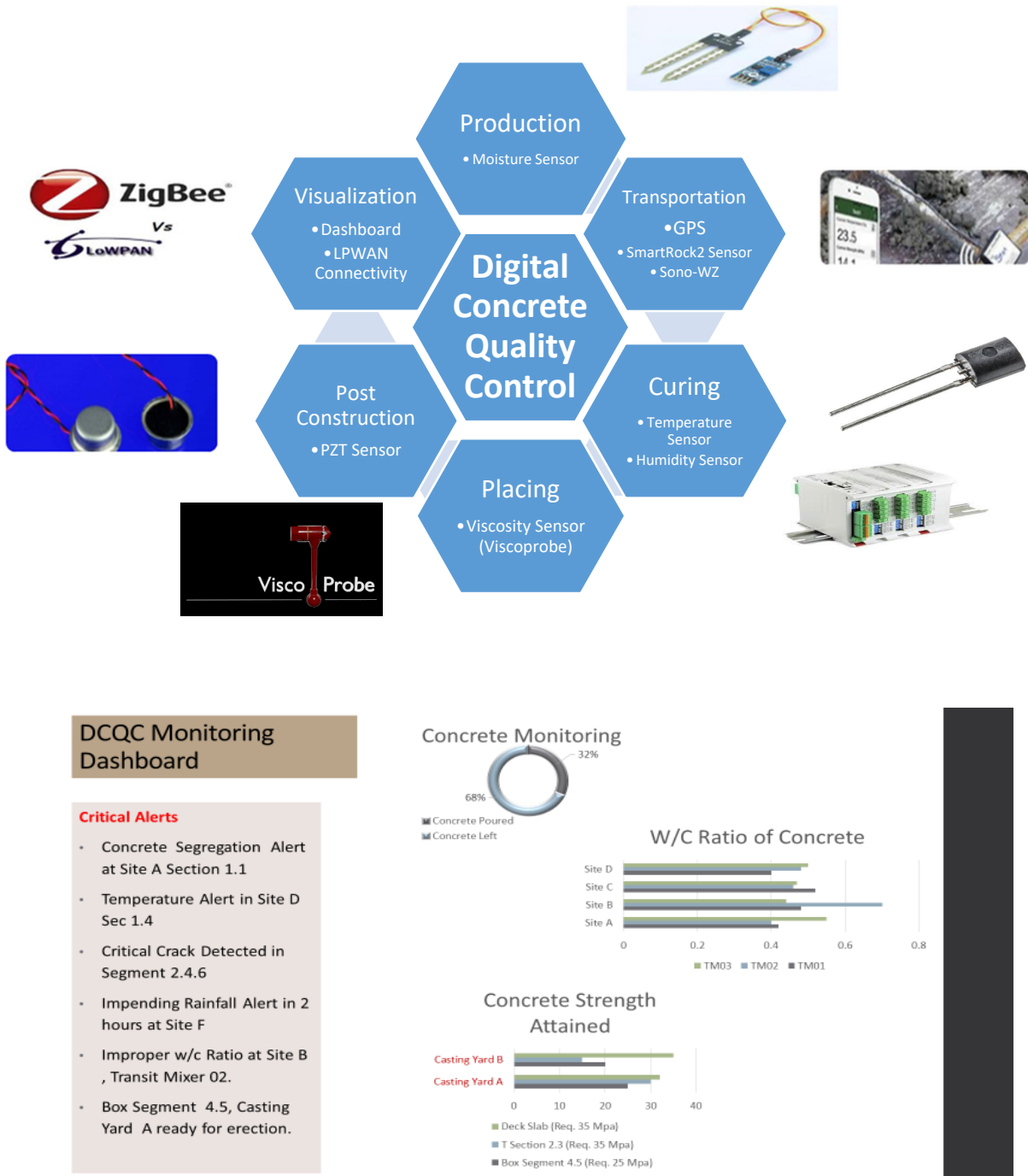
Figure 2. Proposed framework and Dashboard for Digital Concrete Quality Control (DCQC) monitoring
