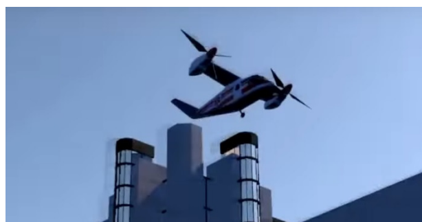
Fig. 3. Tiltrotor aircraft CAT-68 prototype performing corporate flight within the limits of metropolitan area (Source: SPCUV “Virazh” Unmanned Aviation Center)
