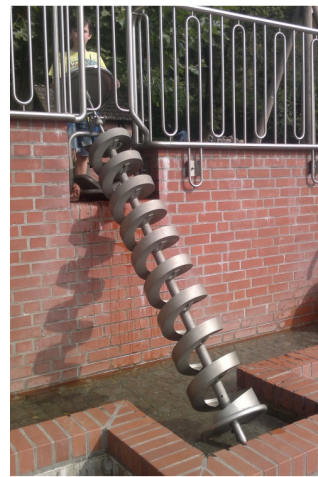
Fig. 3. Principle (Wikipedia 2016) and model of an Archimedean Screw
