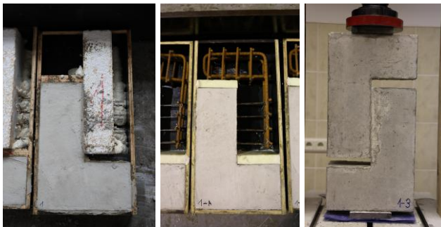
Fig. 3.4. Push-off shear specimen construction process
