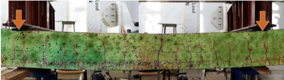
Fig. 3.24. Cracking pattern of slab S-1
