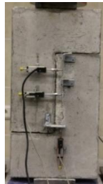
Fig. 3.7. Complete specimen P, L1, and L2 interface failure
