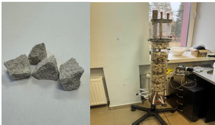
Fig. 2.4. FeCO 3 -impregnated CLC waste particles and the filled biofilter
