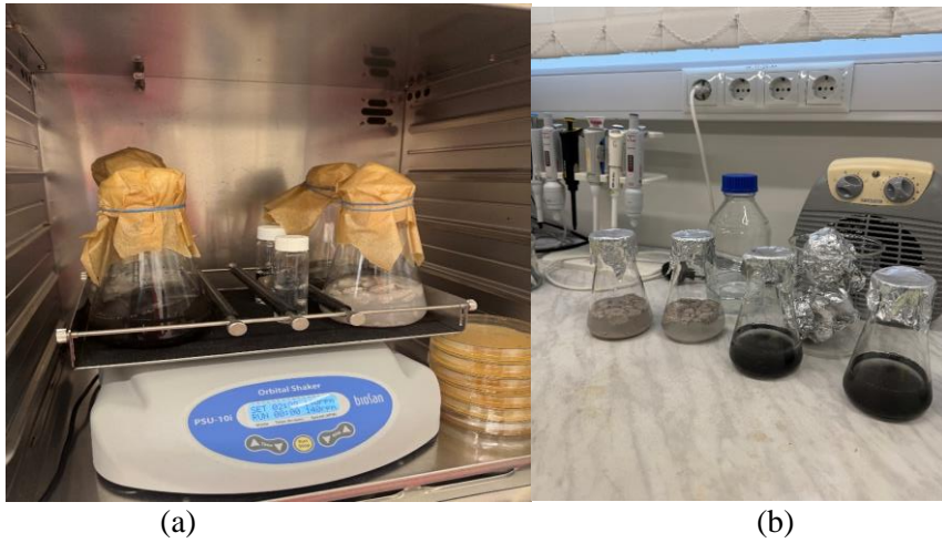
Fig. 2.10. Packing material samples (a) immersed in prepared microbial solutions (b)
