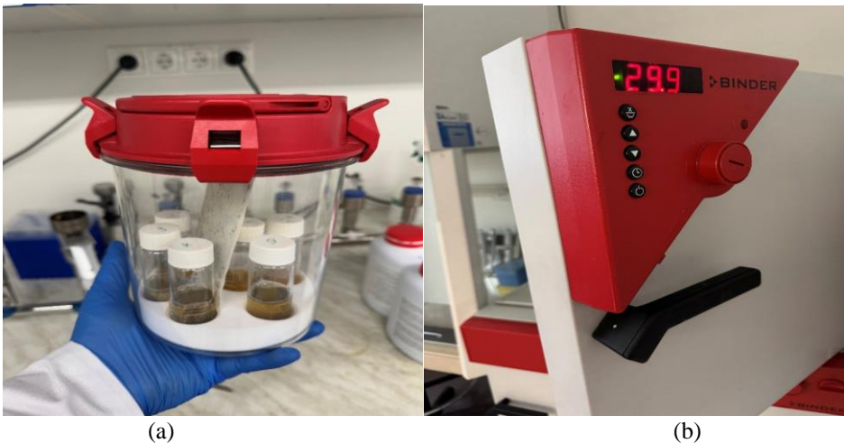
Fig. 2.11. Packing material samples incubated in sealed anaerobic columns (a) and in an oven (b)
