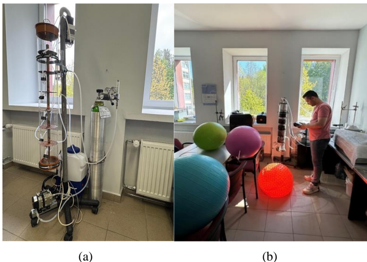
Fig. 2.1. Modified vertical biofilter system used for microbial colonization and \text{H}_2\text{S} purification experiments (a), measuring the chemical composition of injected biogas into the biofilter packed with biochar (b)
