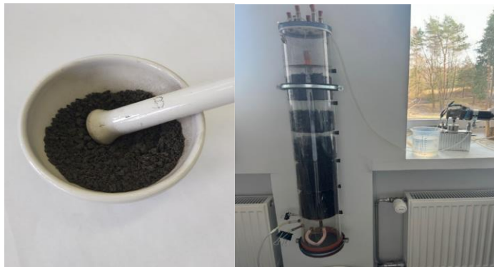
Fig. 2.2. Biochar particles and filled-out biofilter
