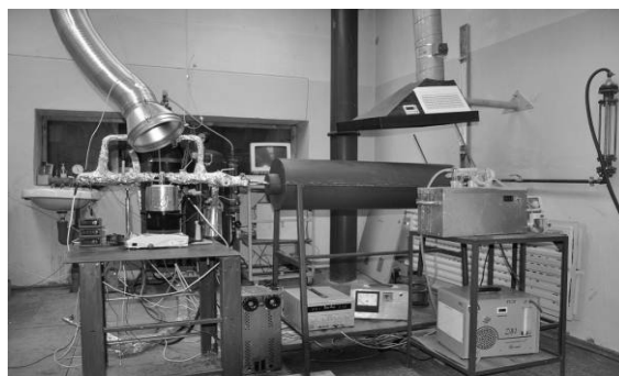
Fig 1. Scheme and photo of the experimental rig: 1 – rotameter; 2 – heater; 3 – water evaporator; 4 – model tar evaporator; 5 – peristaltic pump; 6 – gas washing bottles; 7 – heated bath; 8 – cooled bath; 9 – gas flowmeter; 10 – catalytic bed; 11 – reactor
