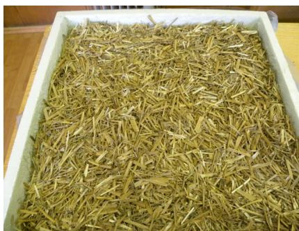
Fig 4. Specimen - 4 for thermal conductivity made from chopped straw
