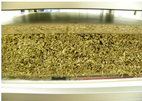
Fig 3. Specimen - 3 for thermal conductivity made from perpendicularly oriented straw to the heat flow
