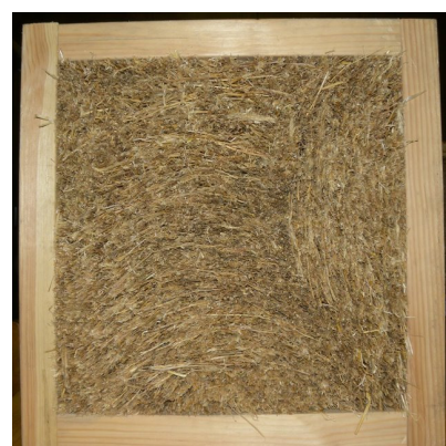
Fig 2. Specimen – 2 for thermal conductivity made from straw roll
