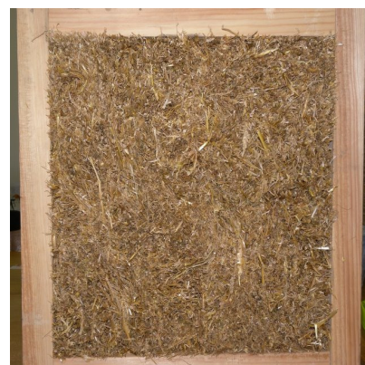
Fig 1. Specimen - 1 for thermal conductivity made from straw bale
