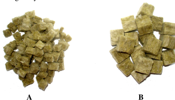
Fig 1. The stonewool substrate: A – 1x1x1 cm cubes, B – 2x2x2 cm cubes
