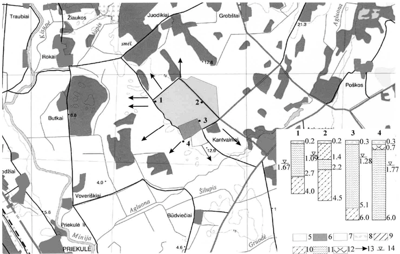
Fig 1. Scheme of the investigation object: 1 - 4 groundwater observation boreholes and their soil profiles; 5 – fields, watered with slurry; 6 – slurry reservoirs; 7 – pig-houses; 8 – plant layer of the soil; 9 – sandy loam; 10 – priemolis; 11 – sand; 12 – peat; 13 – direction of the groundwater flow; 14 – aquifer level
