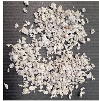
Figure 1. Air dry PMS grains used for this study
