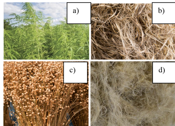
Figure 1. Commonly used bast fibers: a) hemp plant; b) hemp fibre; c) flax plant; d) flax fibre
