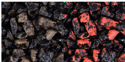
Figure 3. Results of the boiling tests using limestone and gabbro aggregates (13) quartzite aggregate with O-PGB liquid binder (HMA) – 84.8% residual binder coverage (left – image before segmentation, right – image after segmentation)
