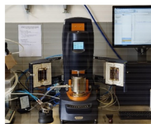
Figure 1. Dynamic shear rheometer with a concentric cylinder accessory used for evaluation of dynamic viscosity of the asphalt binders
