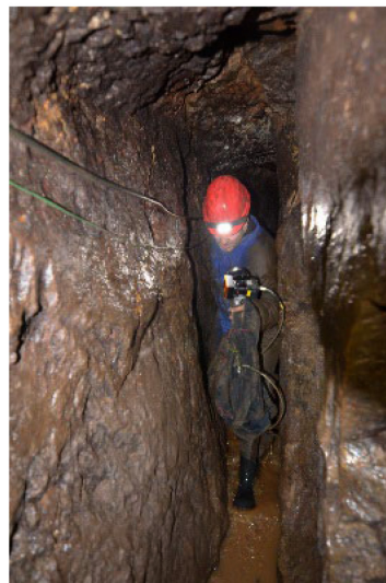
Figure 17. Measurement with PLS is very difficult, confined spaces, running water, dampness, and darkness
