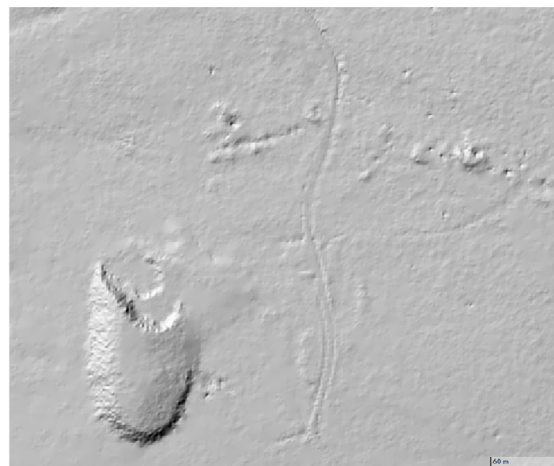
Figure 12. ALS data, Czech state DMR5G model, Eastern Abertamy region, open pits from medieval time (tin mining) and the big deposit from sixties of last century (uranium mining)
