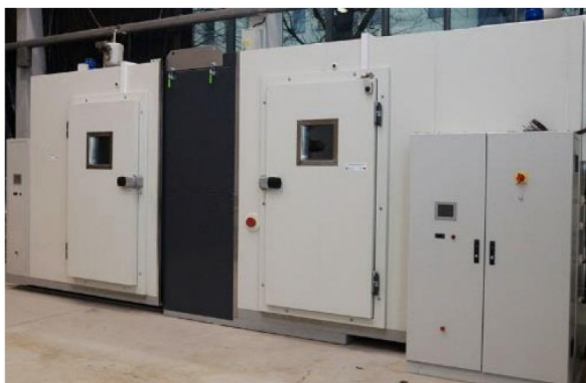
Figure 1. The dual-zone climatic chamber located at the Laboratory of Energy-Efficient Technologies
