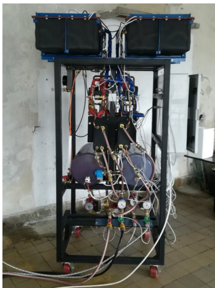
Figure 4. Silica gel-water vapor adsorption system
